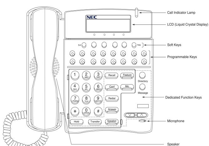
D<sup>term</sup>16D and D<sup>term</sup>16D IP (16-LINE WITH DISPLAY)
